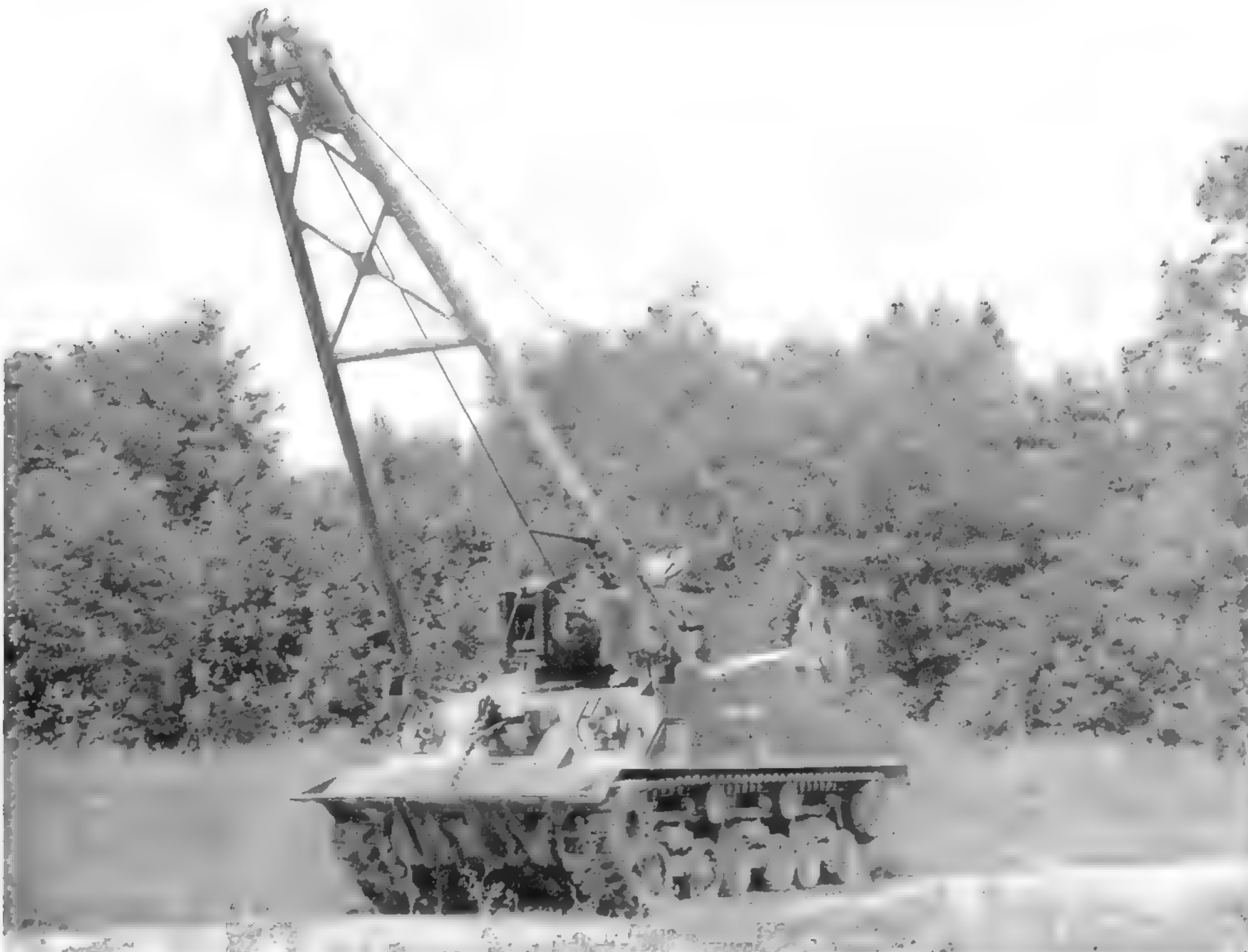
Rather than the windlass arrangement used on the M32 to raise the A-frame, the M74 used hydraulically actuated rigging. In addition to being simpler to operate, the M74 had an A-frame that could be used as a live boom, being raised and lowered while under load. (U.S. Army photo)
